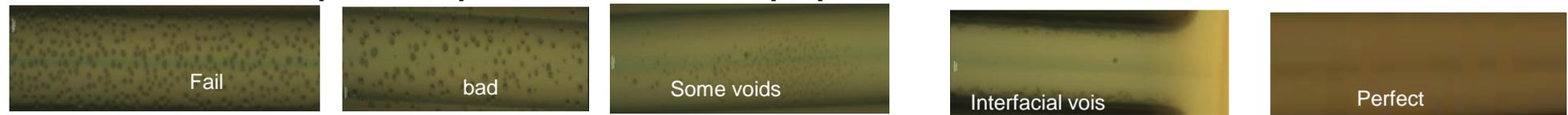
High resolution microscopy images of waveguide with optical adhesive
