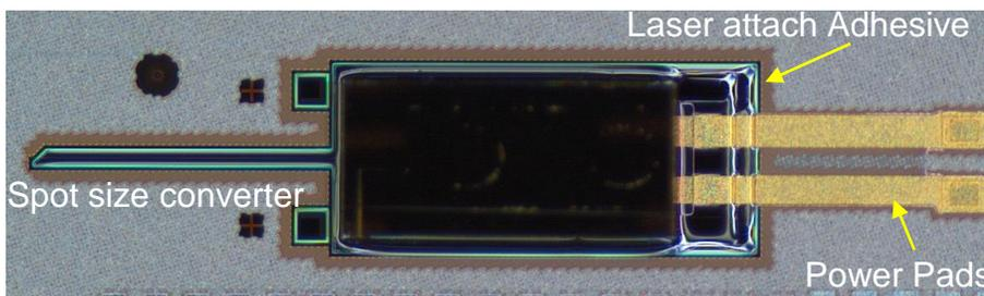
Assembly of a III-V Laser into a Silicon Photonics Cavity
