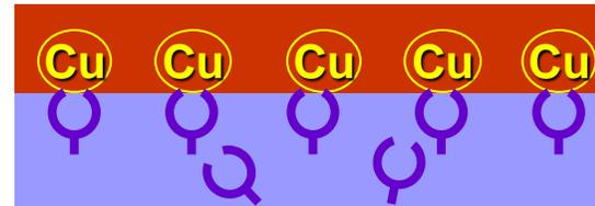
Thin Cu works for self-assembly of specific bonds on the resin surface and as a protective layer against desmear.
