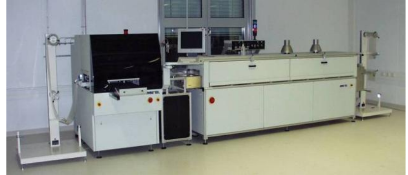
Thick-film screen printing on sheets and rolls
