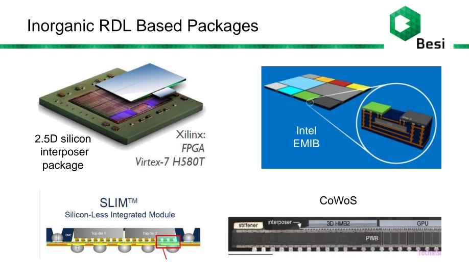
Based on inorganic RDL (silicon oxide, silicon nitride)
