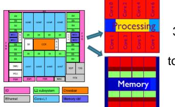
3D-SOC Study for OpenSPARC T2 to be 3D-integrated into Logic + Memory
